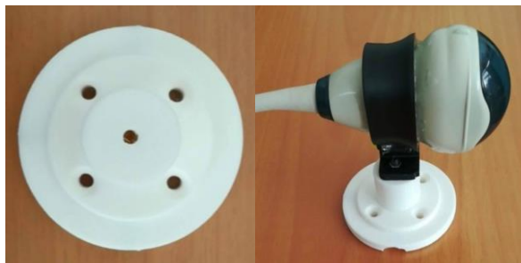
Figure 6 - Picture of the 3D printed holder and its assembly to the US probe hoop (on the right).
